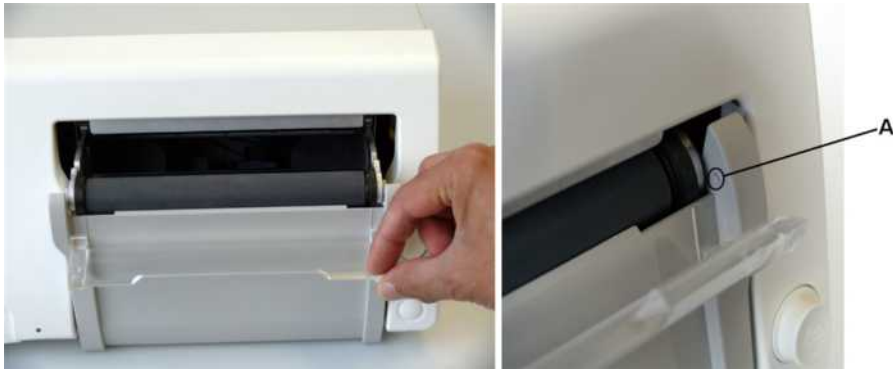
A - Protrusion holds paper guide in closed position
