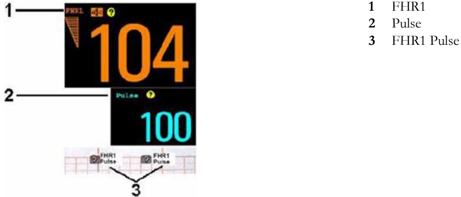
Avalon CCV numeric display and recorded trace showing coincident alerts
